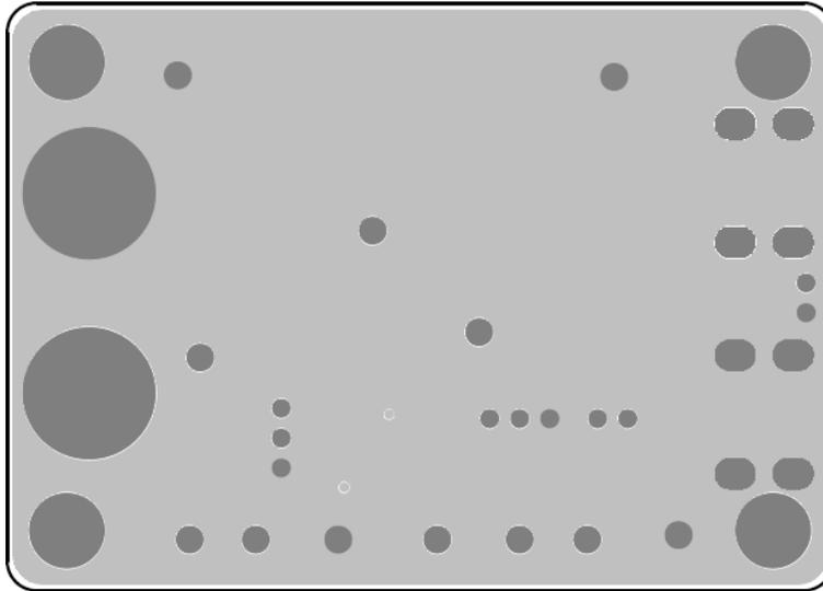
PCB Layout—Inner Side (3<sup>rd</sup> Layer)
